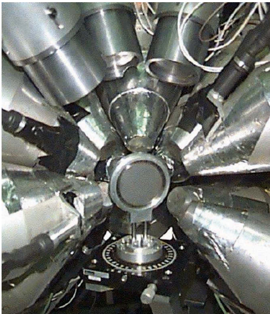
Figure 4. The GEANIE Detector GEANIE is composed of 26 high-purity germanium detectors. The photo shows them viewing gamma rays from an encapsulated plutonium-239 sample bombarded with neutrons from the WNR source.
