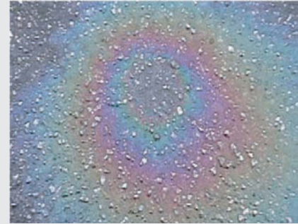
Figure A. Reflections from an Oil Film on Water The varying thickness of the oil film creates rings of color.
