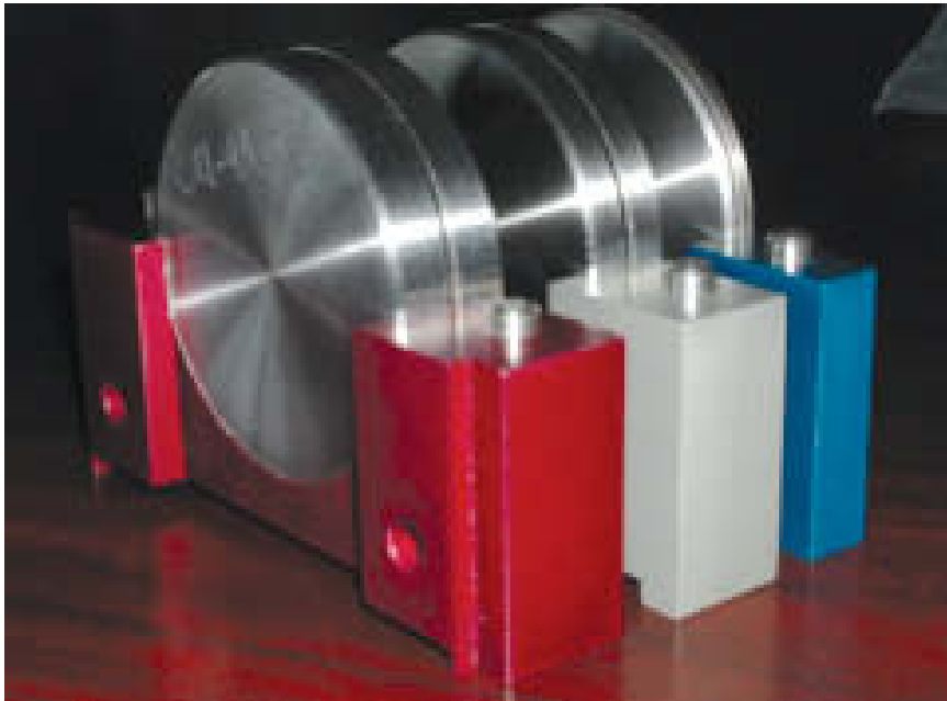
Figure 4. Target Stack and Carrier Disc-shaped targets of varying thicknesses and compositions are placed in the carrier (shown here without its upper part). The protons travel from left to right through the target stack and lose energy as they undergo Coulomb scattering in the target materials. Protons strike the first (leftmost), second, and third targets in the stack with nominal energies of approximately 90, 65, and 40 MeV, respectively.
